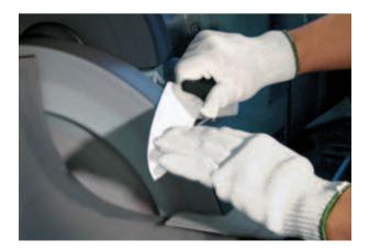
Sharpening is performed on either a sharpening stone or a polishing wheel. The cutting angle is checked using a laser.
